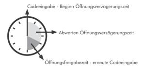
It allows delay times of 1 to 99 minutes and release times of 1 to 19 minutes to be set. An opening time that has been started can be stopped by pressing any key.
