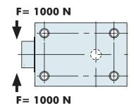
• The load on the bolt must not exceed 1000 N.
