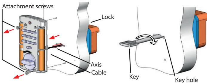
Depending on the type of mounting, the cable has been run through the axis (see image on page 29) or through a separate drilled hole.
