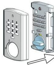
After the cover has been installed, the key tones will sound deeper until a valid code has been entered. If, despite the correct mounting of the cover, you hear deep tones, check the keyboard for possible tampering!
