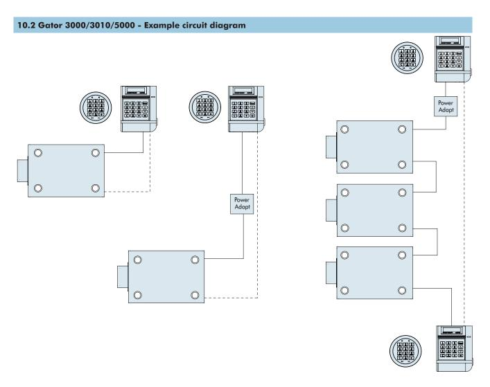
\_\_\_\_ optional bus cables for redundancy
