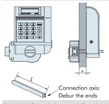
L = A + 48 mm (tolerance -1,5 mm)
