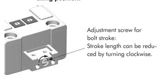
• Gator 5000/6000/8000/9000: Stroke length can be be adjusted continuously from 9 – 15 mm (factory mode: 15 mm).
