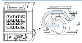
• Lead connection cable through the connection axis and input unit.
