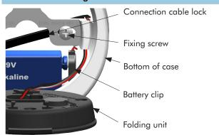
• Lead connection cable lock and connection cable battery behind the bottom of casse of the input unit..
