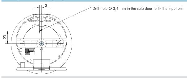
• Fit input unit of approx. 20° (see 3.5.2), adjusting to the locked lock/boltwork and insert grub screw M3 x 6 or arrest pin.
