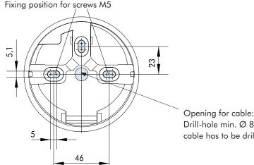
Opening for cable: Drill-hole min. Ø 8 mm/max. Ø 11,4 mm for connection cable has to be drilled into the safe door
