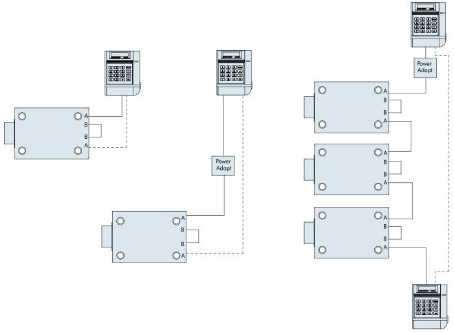
\_\_\_\_ optional bus cables for redundancy
