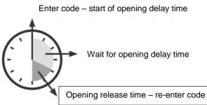
It allows delay times of 1 to 99 minutes and release times of 1 to 19 minutes to be set. An opening time that has been started can be stopped by pressing any key.
