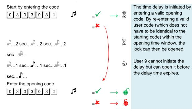
If the dual code / "four eyes" principle is enabled, the opening process corresponds to the opening process described at the end of the time delay.
